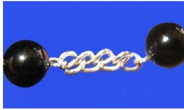
Traditional chain for Rosaries is attractive and strong. Each link consists of two loops. The wire used here is 0.7mm silver plated brass. The chain and Rosary are made at the same time. Success depends on the wire for each new loop passing through the previous link/loop in the right direction. Otherwise the new link will be formed backwards and the chain fail.
