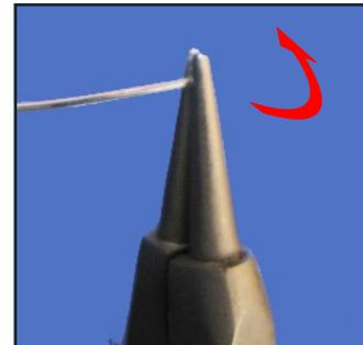
2. Rotate the pliers away from you while, at the same time, with the other hand, bend the wire around the plier also away from you. This will produce a **P** shape loop.
