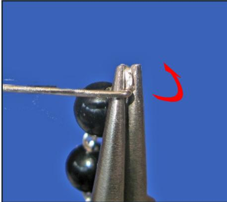
5. Rotate the pliers away from you while, at the same time, with the other hand, bend the wire around the plier also away from you.
